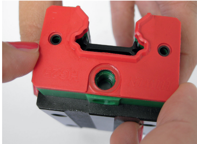
Fig. 12: Placing of the end seal
